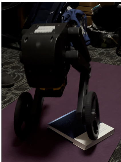
Figure 5: Rhea Successfully Traversing a Ledge, Using the RL Controller
