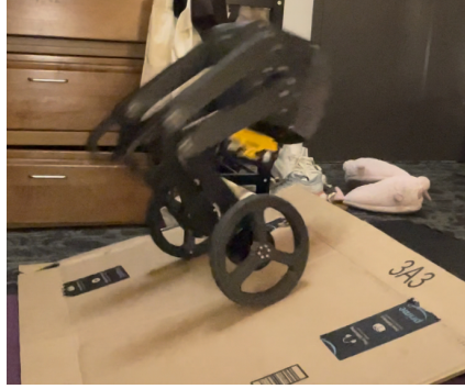
Figure 6: Rhea Successfully Scaling the Ramp, Using the RL Controller
